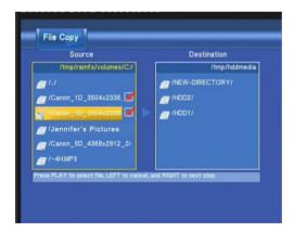
(4) Now press the right navigation button in order to select the "Destination" column. Select the directory the files will be transferred to. Once selected, press the right navigation button to proceed to the next step.
